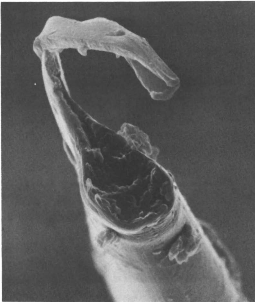
Figure 5. SEM photomicrograph of a Type 7 (surface-flaw-influenced) fracture (2600 \times ).
