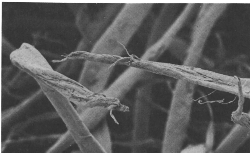
Figure 12b. Cotton fibers present in a worn portion of a used cotton-polyester sock (572 \times ).
