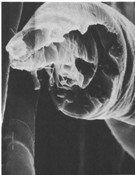
Figure 20. Scanning electron micrograph of a cotton fiber aged at 190 °C under conditions of LO (8,640 \times ).
