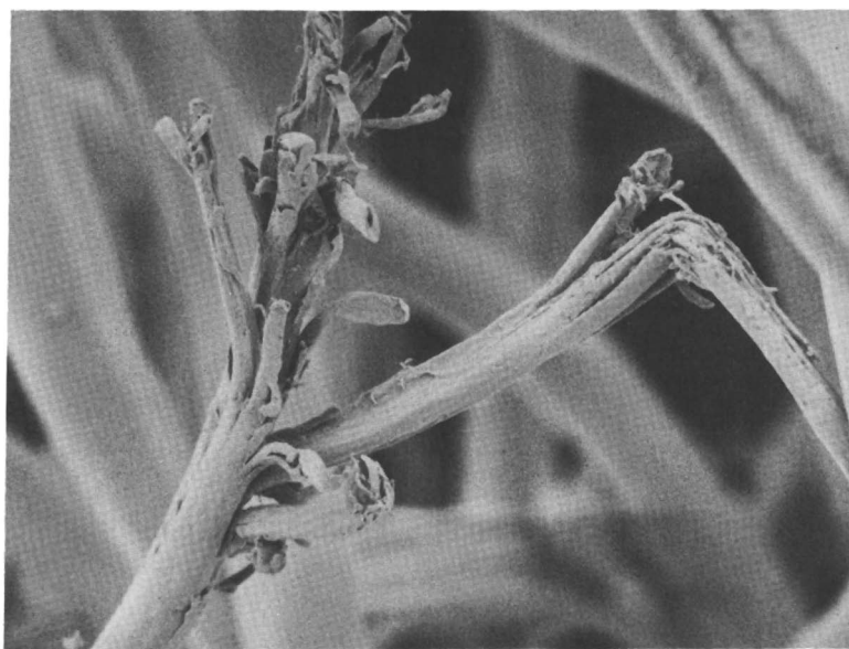
Figure 12a. Cotton fibers present in a worn portion of a used cotton-polyester sock (617 \times ).
