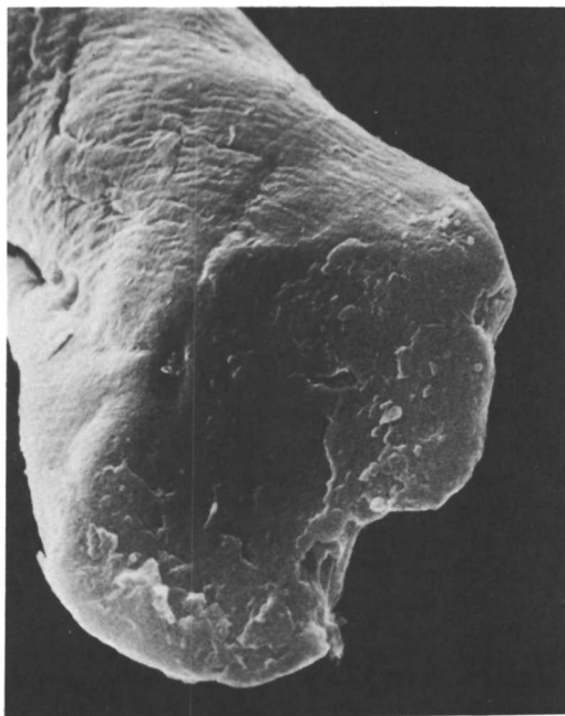
Figure 21. Scanning electron micrograph of a cotton fiber aged at 190 °C under conditions of LN (8,480X).
